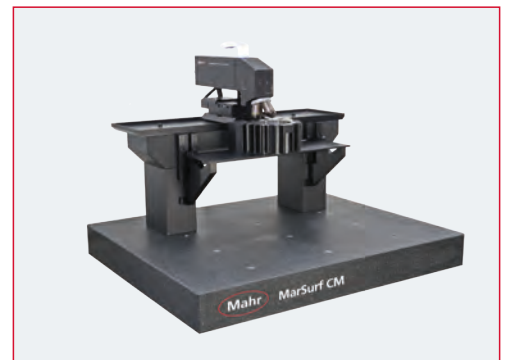
A specially adapted stationary work station allows large, heavy test objects to be put down.
