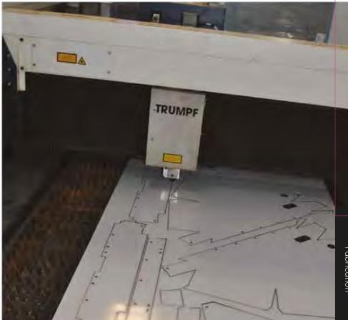
The processes available for metal cutting include laser cutting, plasma cutting, water jet cutting, punching, stamping, and hard material cutting using electric discharge machines (EDMs). In terms of metal forming, Omnidex offers a range of bending, shearing, deep drawing, roll forming, spinning and welding services.
