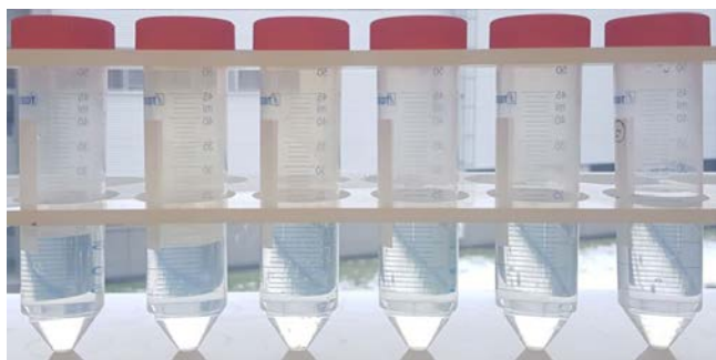
Figure 5: Digestion solutions, Multiwave 5000 (left to right: raw milk, butter, yoghurt with fruits, cottage cheese, curd, skimmed milk powder)
