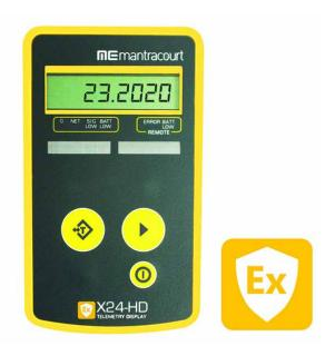
The X24-HD ATEX wireless portable display has approvals for hazardous zones 1 and 2 and allows remote viewing of multiple X24 ATEX and T24 wireless transmitters. This handheld ATEX display is compact and portable delivering easy on-site monitoring, with a range of up to 1/2 mile (800m).
